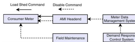
Figure 4: AMI control functions (Sridhar et al., 2011).
